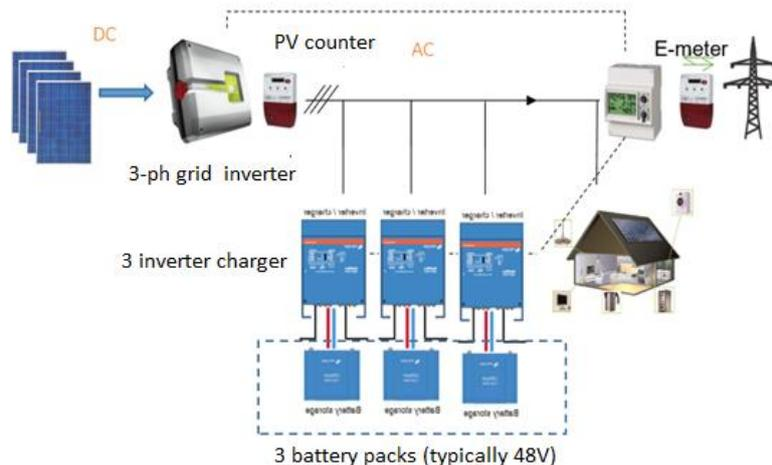
Figure 2. Example medium/large PV system. Source: KOSTAL.
